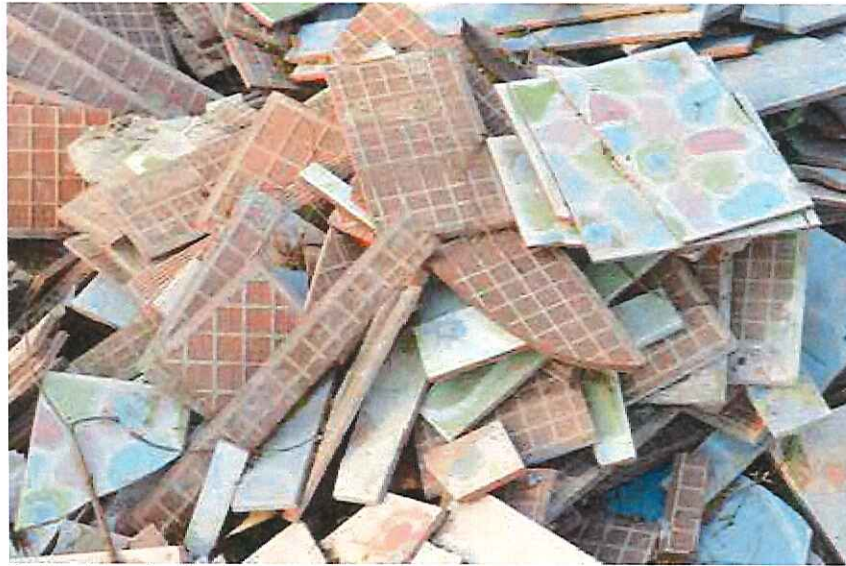
Broken asbestos floor tiles
