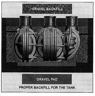
Cover all openings, then begin backfilling with gravel under and around the sloped clarifier. Continue to add gravel until the discharge line from the Singulair Green tank is covered. Proceed to the inlet end of the pretreatment chamber and add gravel until the inlet line is covered. Fine, loose earth may be used to backfill the remainder of the excavation.
