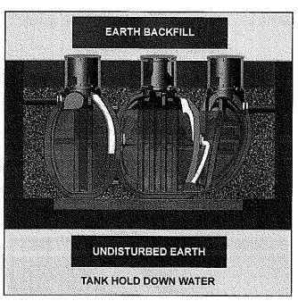
When pumping or dewatering the Singulair Green tank, only pump the pretreatment chamber. Then, promptly refill the tank to capacity with clean water. Dewatering and leaving the Singulair Green tank empty will effect tank integrity and void the Singulair Green warranty.
