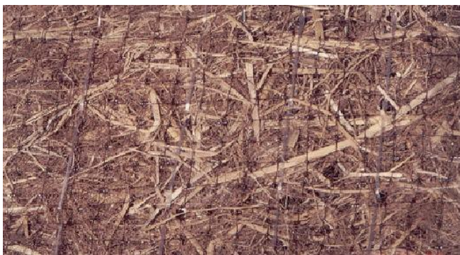
Straw Matting (photo courtesy of Clean Water Services)
