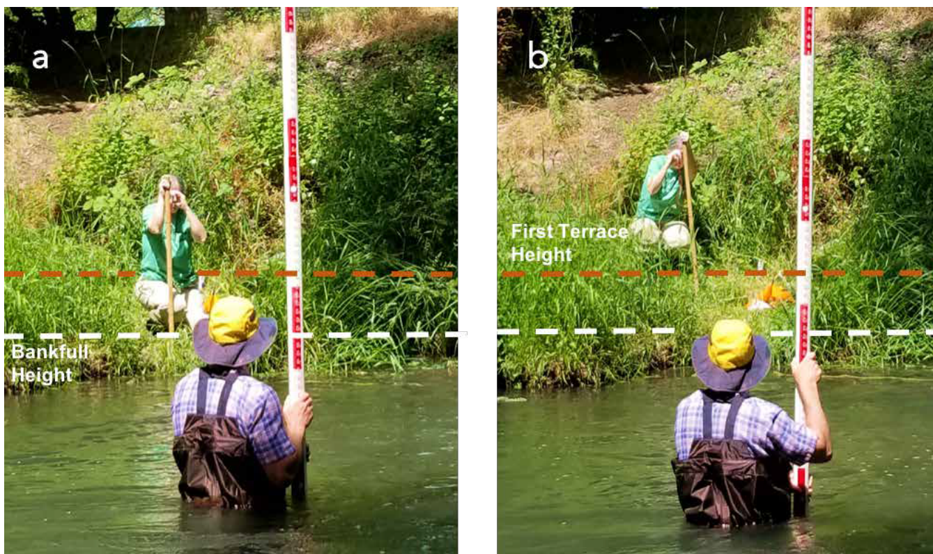
Figure 5.18 Using a clinometer to site the bankfull height (a) and the first terrace of the valley floodplain (b).
