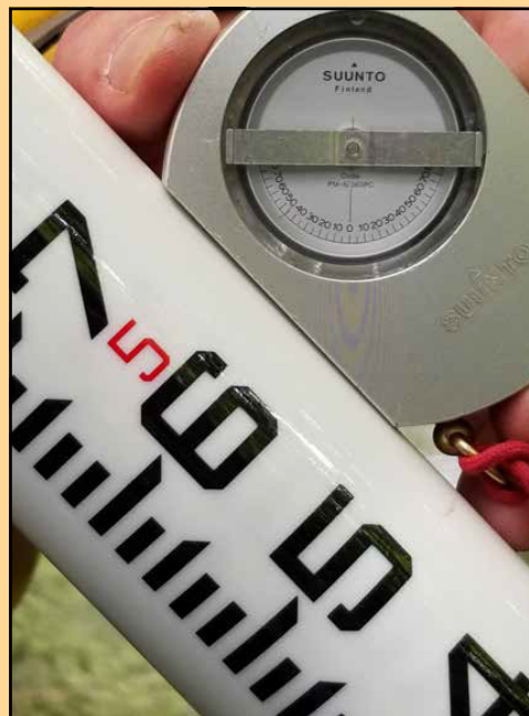
Figure 5.21 Using a clinometer to hold a stadia rod at a 45-degree angle.
