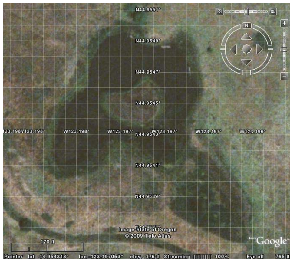
Figure 4. Using Google Earth© with the grid feature to generate potential sampling locations. Each grid within a habitat class could be numbered, and each corner of a grid could be a potential sampling location. Both the grid number and the corner could then be randomly selected.
