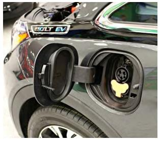
station, and several manufacturers of charging equipment now manufacture dual-standard equipment. Electrify America has committed to installing both of these standards at all DCFC stations they build.
