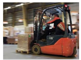
Electric battery forklift. Photo: Toyota Material Handling
