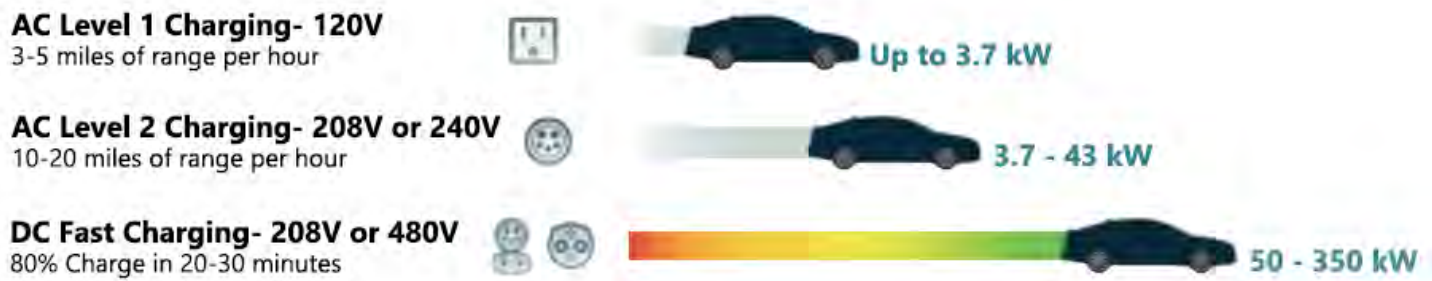
Figure 2: Level Up: Peak Demand of Different EV Chargers 4
