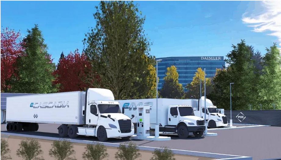
“Electric Island,” a joint project by Portland General Electric and Daimler Trucks North America is a first-of-its-kind electric fueling station capable of charging everything from light-duty passenger vehicles to electric freight trucks. 62
