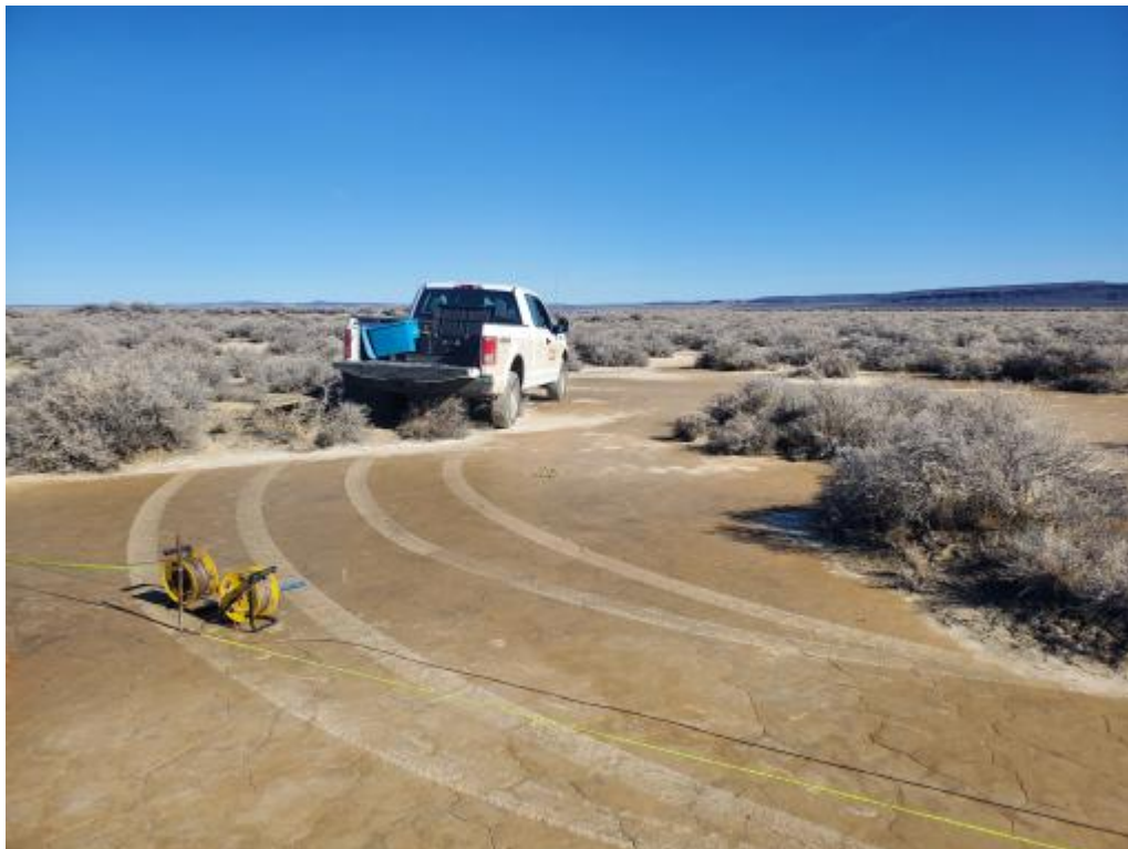
Photo 6: Electrical resistivity testing activities
