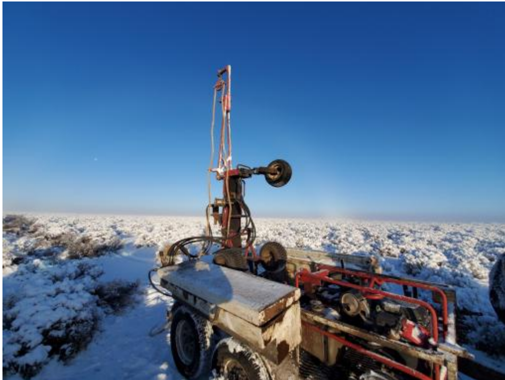
Photo 3: Truck-mounted drill rig used for exploration
