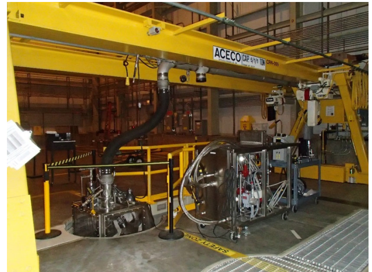
MCO sampling for gaseous constituents, gas pressure, and temperature (Covert 2017)
