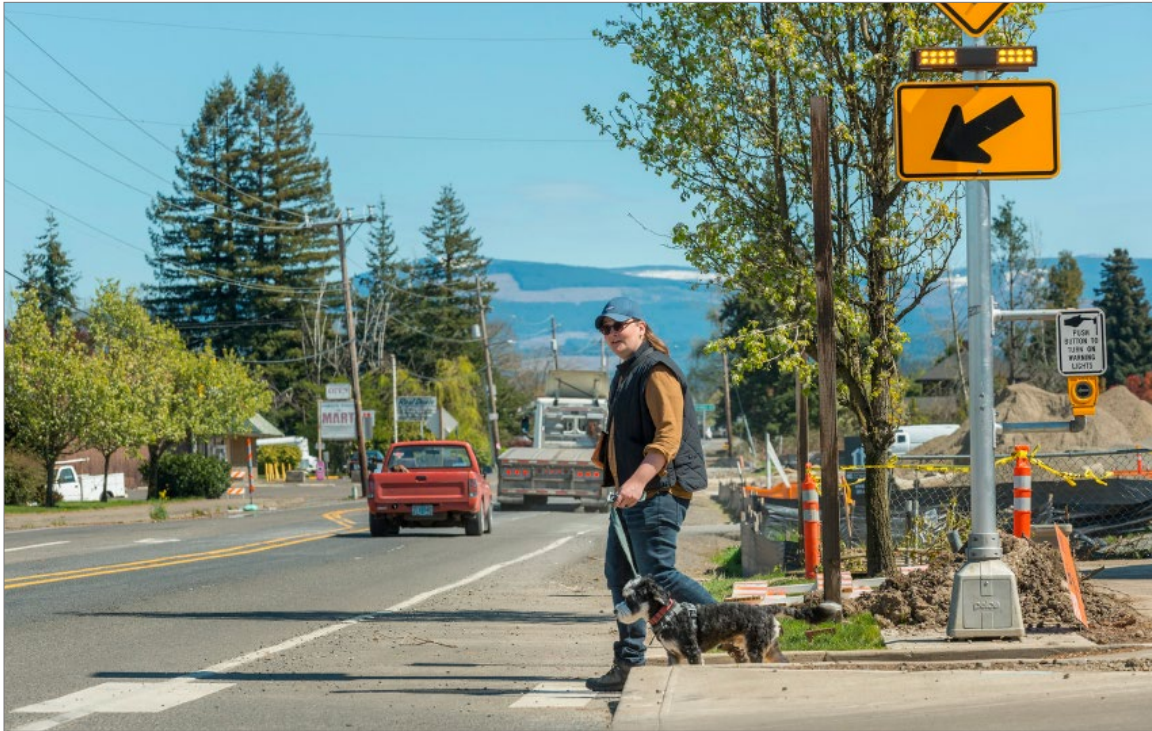
Pedestrian flashing beacon and crossing | Source: ODOT
