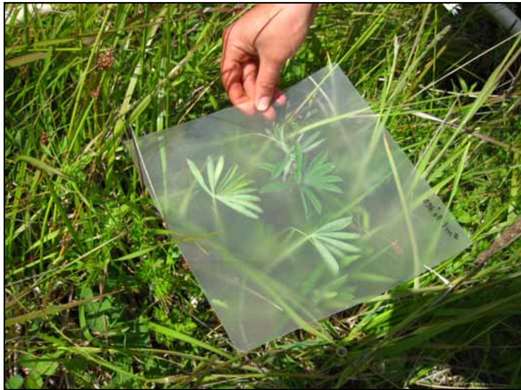
Figure 11. A transparent or semi-transparent square measuring 22.36 cm x 22.36 cm (representing 5% of a square meter or 0.05 m 2 ) can be helpful when estimating area cover.
