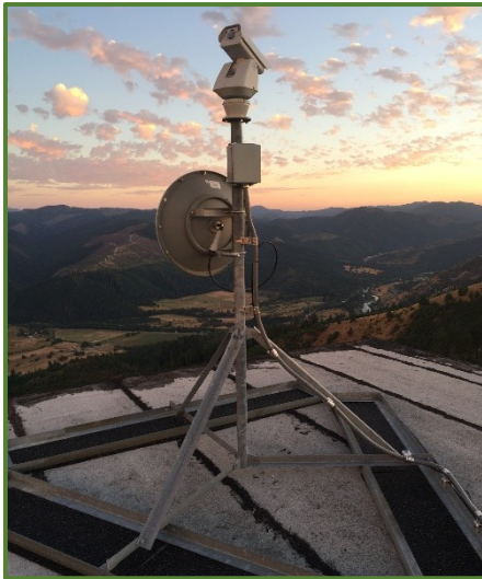
Figure 7. Bland Mountain Smoke Detection Camera
