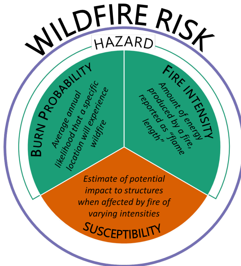
Figure 1. Representation of the three components of wildfire risk to structures. When combined together, burn probability and fire intensity represent wildfire hazard.
