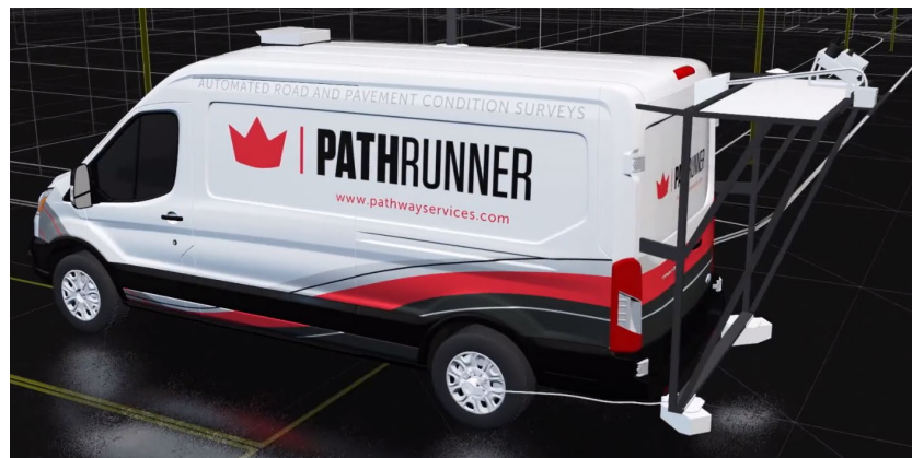
Figure 4 – Pavement Data Collection Vehicle used for Automated Distress Survey
