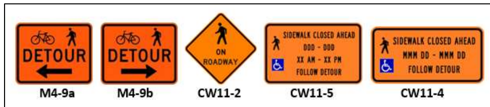
Figure 3-8: Examples of TPAR Guidance Signs
