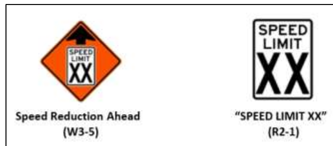
Figure 3-29: Speed Reduction Signs
