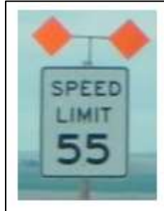
Figure 2-9: Sign Flag Boards on a Speed Limit Sign
