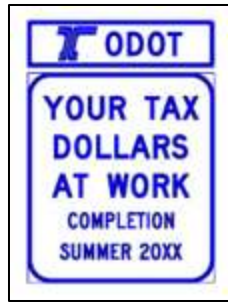
Figure 2-11: Project Identification Sign
