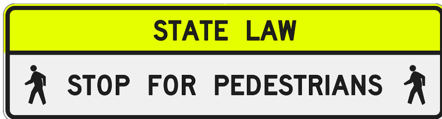
Figure 186: Overhead Pedestrian Crossing Sign (R1-9a)
