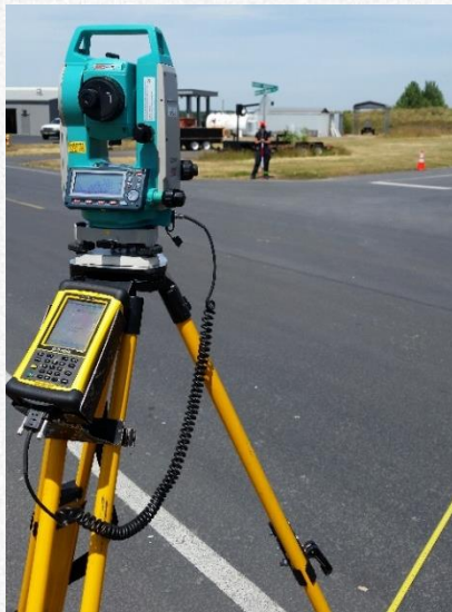
Picture of a Robotic Total Station used to quickly map a crash scene for crash investigation.
