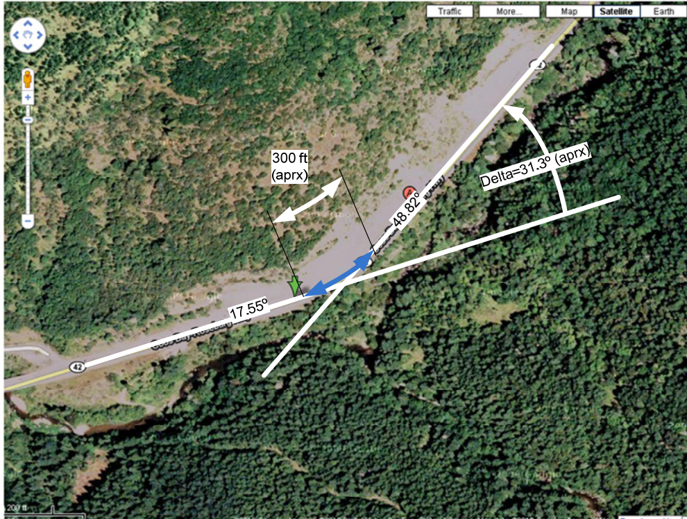
Figure F.2: Deflection Angle and Curve Length Estimation
