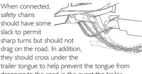
dropping to the road in the event the trailer separates from the tow vehicle.
