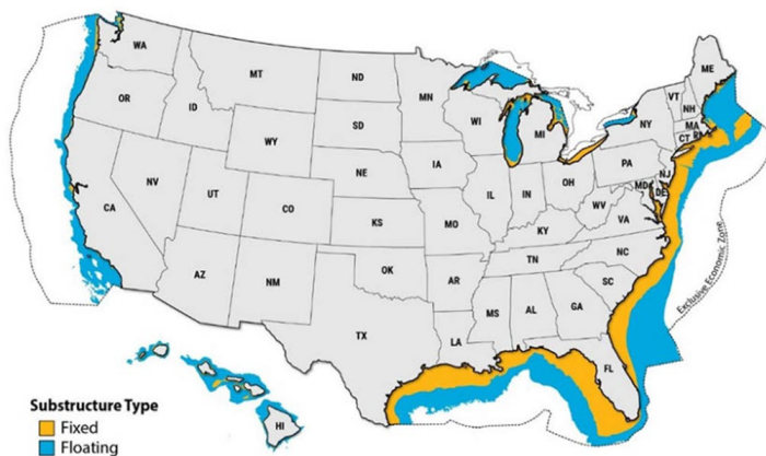
Figure 2. Nationwide offshore wind resources by structure type for the United States (Source: NREL)
