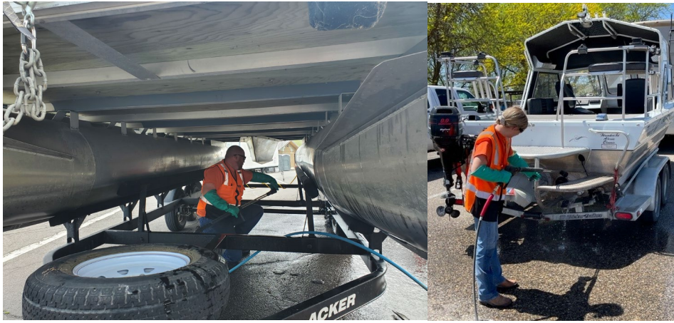
Figure 5 and 6. Two boats intercepted at the Oregon Department of Fish and Wildlife’s watercraft inspection stations; both boats were inspected and attached quagga mussels were found. We decontaminated both boats on-site and re-inspected with no additional mussels found.
