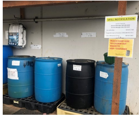
Very organized waste storage area with spill containment pallets. All labeled according to requirements
