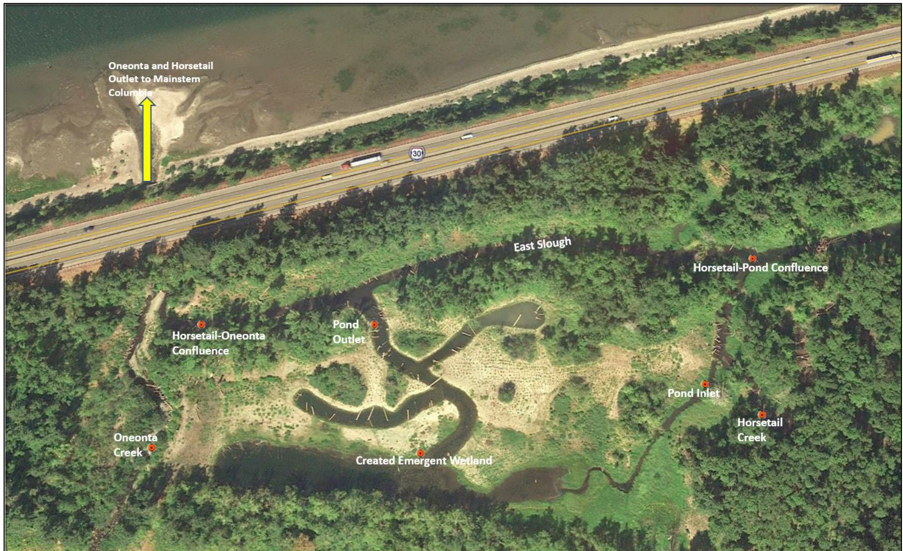
Figure 5: Temperature monitoring locations at Horsetail Creek Floodplain restoration site. Monitoring locations are represented by red dots. The outlet of the I-84 culvert which was retrofitted during construction is shown as the yellow arrow.
