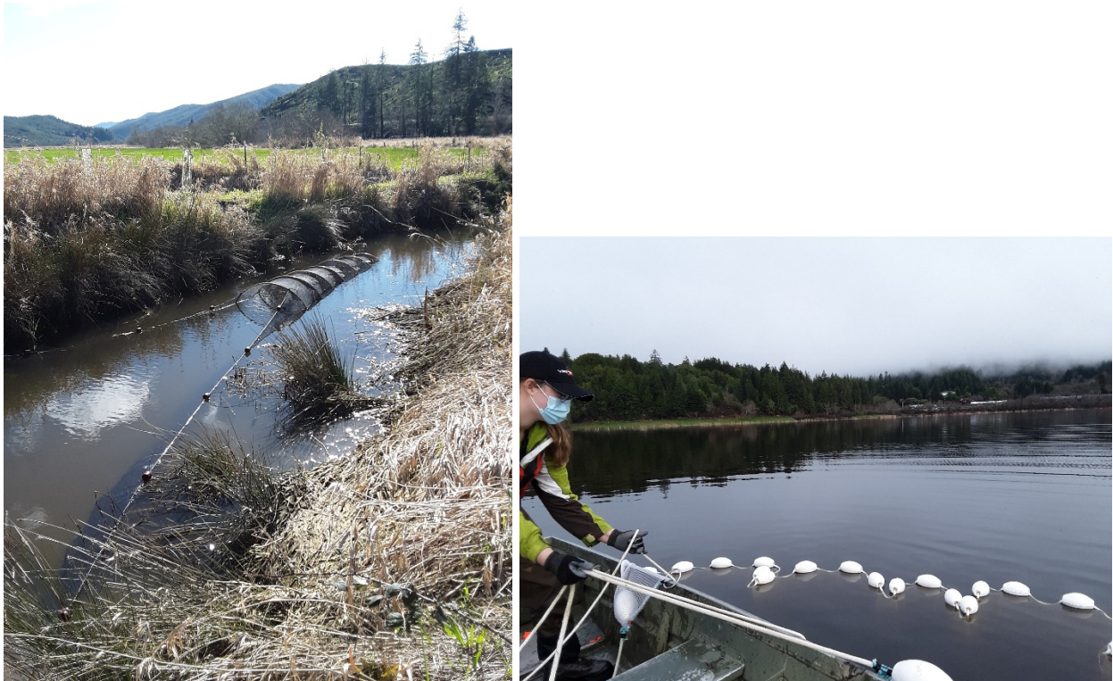
Figure 7. A 4' hoop trap with 25ft leads installed at the Cochran site. Hoop traps were used at most sampling sites in the 2020-2021 field season (left) but only at Cochran, Seestrom and Beaver Slough in the 2021-2022 season. During flood periods a purse seine was used to sample in the flooded project site of Winter Lake (right).
