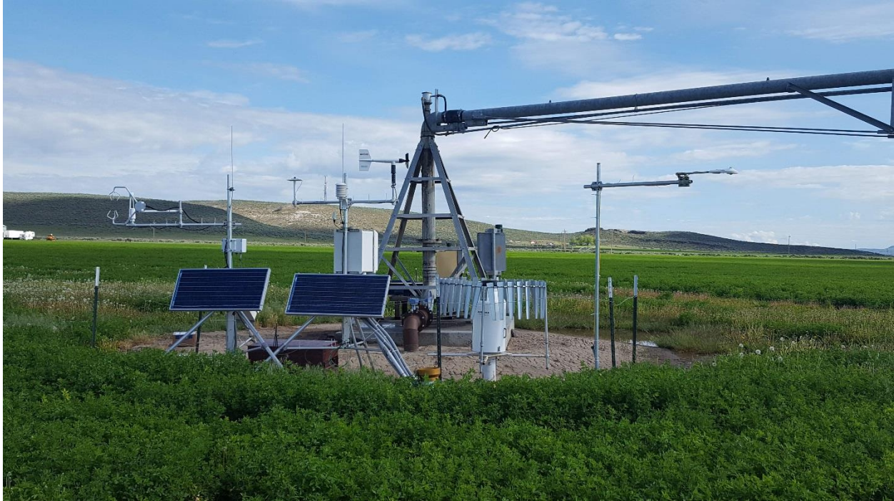
Figure 3. Eddy covariance station (CRN) at groundwater irrigated site, Owens Hay Farm, May 2019.
