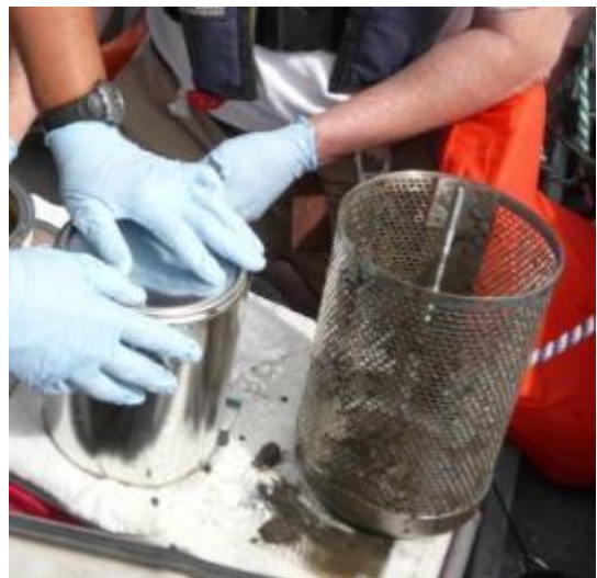
Figure 14. Residual sediment on John Day River SPMD canister.
