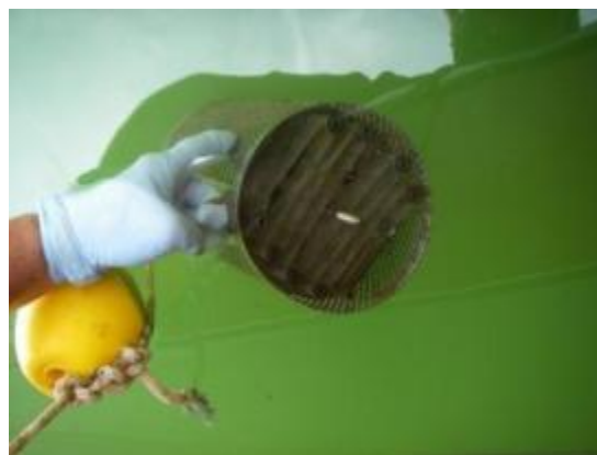
Figure 6. An SPMD canister about to be retrieved. The lid has been removed underwater, revealing the first of five
