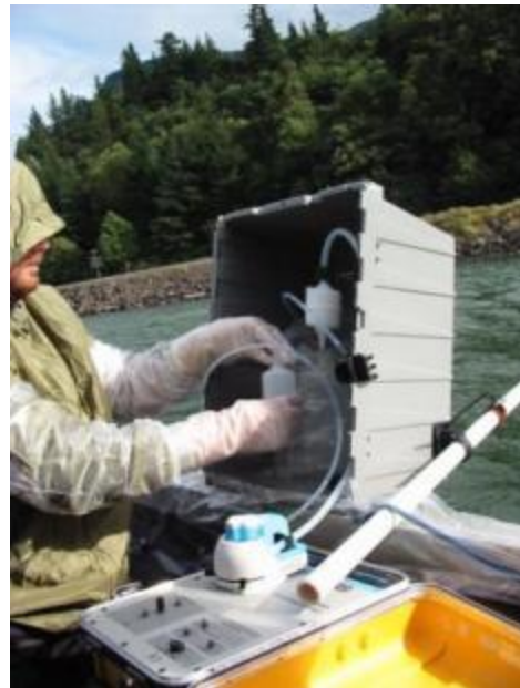
Figure 2. Water samples were collected using EPA Method 1669 for trace
