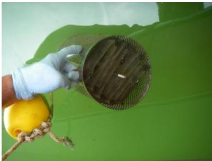
Figure 35. An SPMD canister held below water during retrieval. The end cap has been removed, and the first membrane visibly winds back and forth on the "spider" array. The yellow float held the snag line off the bottom during deployment to facilitate retrieval with a grapple.
