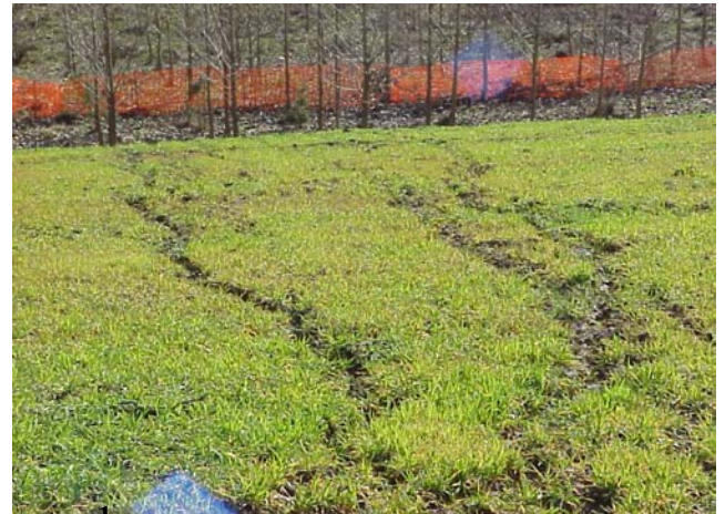
Rills Form on Surface w/out Compost
