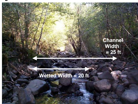
Figure 12.4 Channel width measurement
