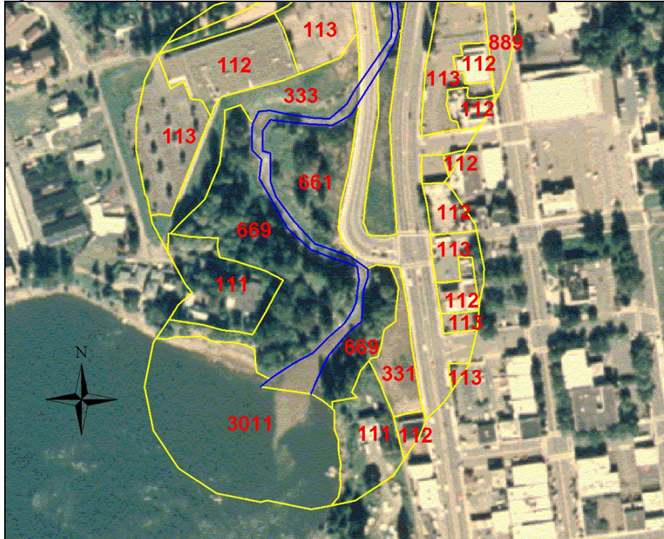
Figure 5.53. Example of Near Stream Land Cover Delineation at the confluence of Johnson Creek and the Willamette River.
