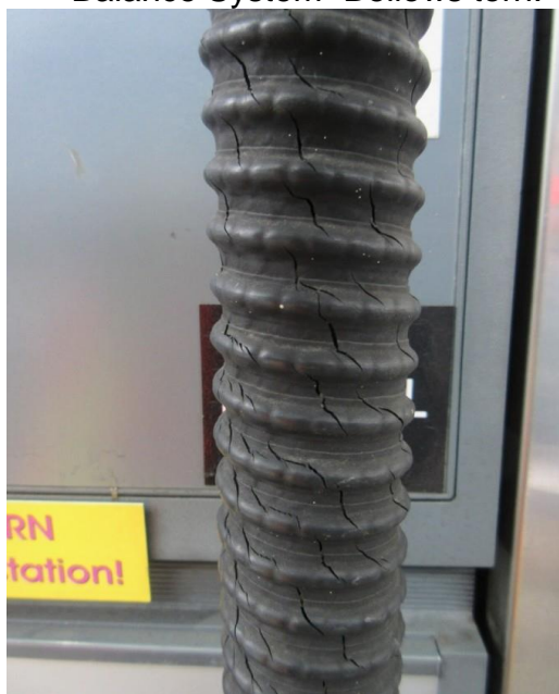
Balance System- Hose tears.
