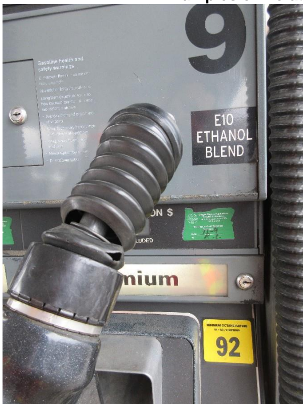
Balance System- Bellows torn.
