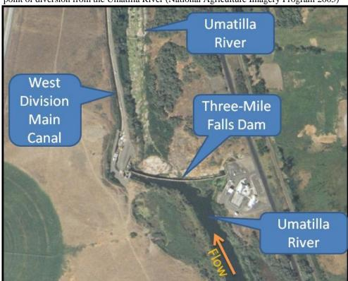
Figure 2. Aerial photograph of Three-Mile Falls Dam and West Division Main Canal point of diversion from the Umatilla River (National Agriculture Imagery Program 2005)<sup>11</sup>
