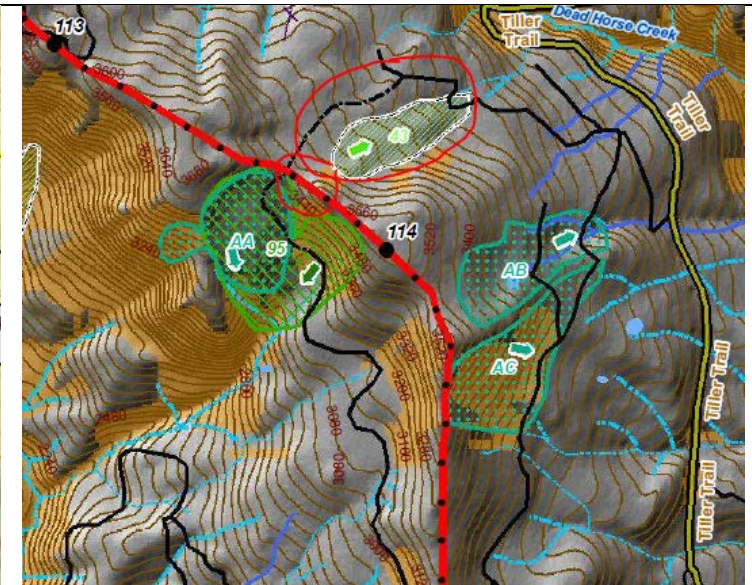
Location of PAR-113.66 and Proposed Road Reconstruction relative to landslide features. Figure 25 of 47. Note: the light brown areas are Potential Rapidly Moving Landslide Hazard
