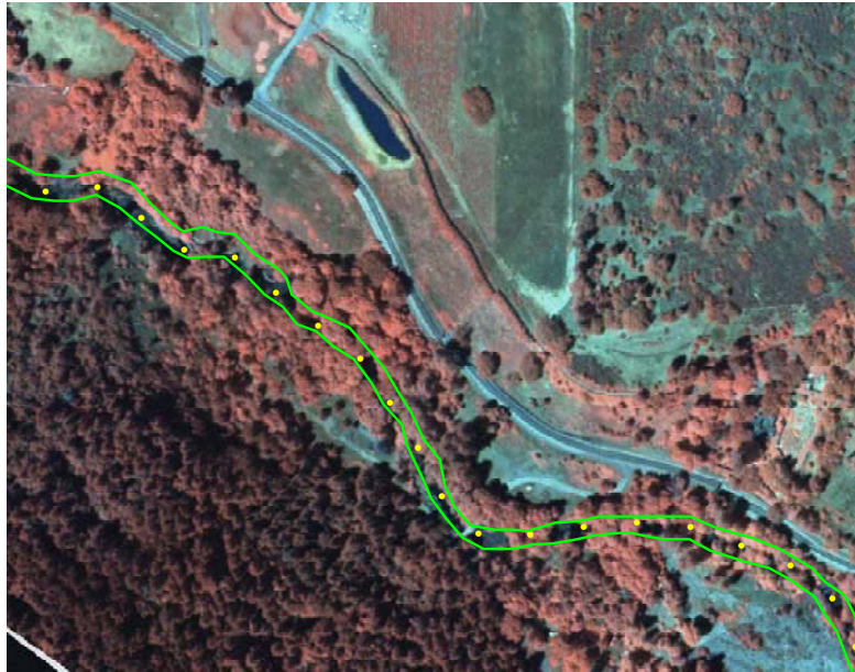
Figure 1-7: Near Stream Disturbance Zone Drawn on Photo. A GIS utility is then used to measure this distance at each segment break.
